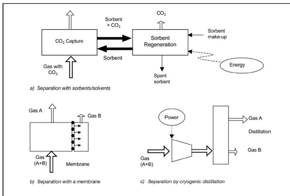
**Figure 8 Technological options for Carbon capture and utilization**
