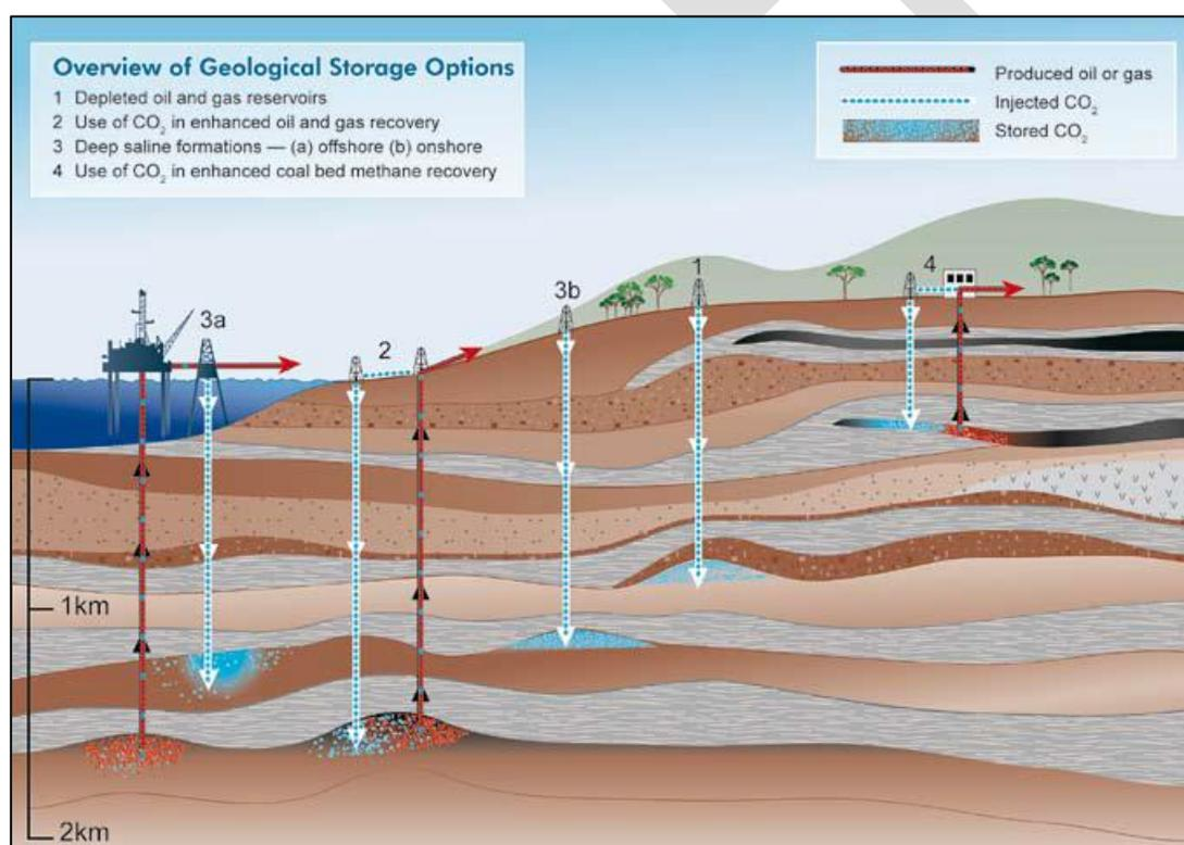
**Figure 9 Typical CO<sub>2</sub> storage illustration (Source: Carbon Capture and Storage, IPCC Report, 2005)**
