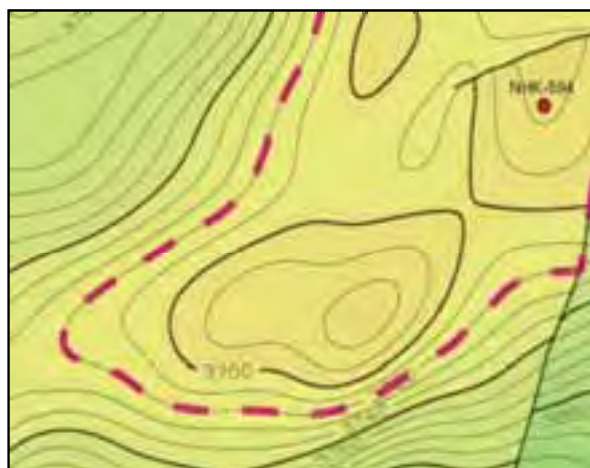
Kharikatia Structure with well NHK-594 – Depth Contour Map Close to Langpar Top
