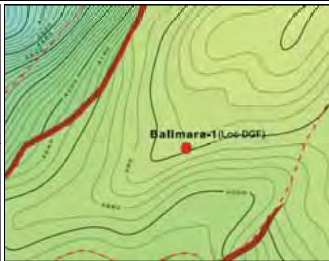
Balimara Structure with well Balimara-1 - Depth Contour Map Close to 34 SB / Near Top Barail
