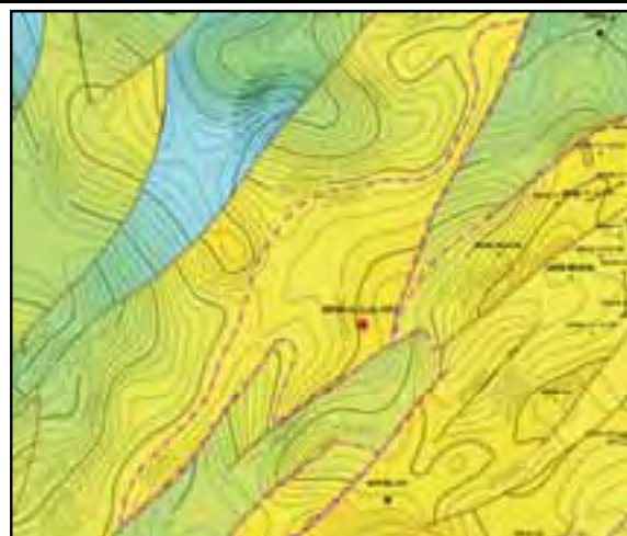
NW Makum Structure with well MKM-41 – Depth Contour Map Close to 34mfs/Near Top Barail 3/4
