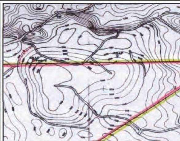
Punam structure with well Punam-1 Depth Contour Map on top of Jodhpur S.St.
