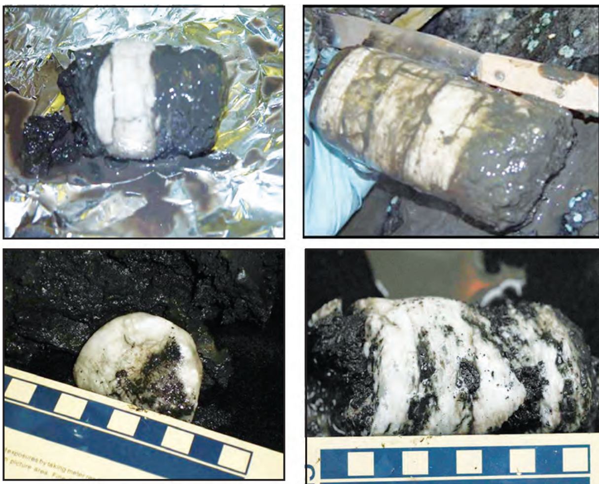
GAS HYDRATE CORE SAMPLES FROM KG BASIN – EXPEDITION-01
