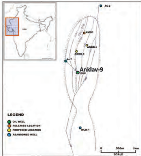
Structure Contour Map On Top of EP-Ib Pay Sand
