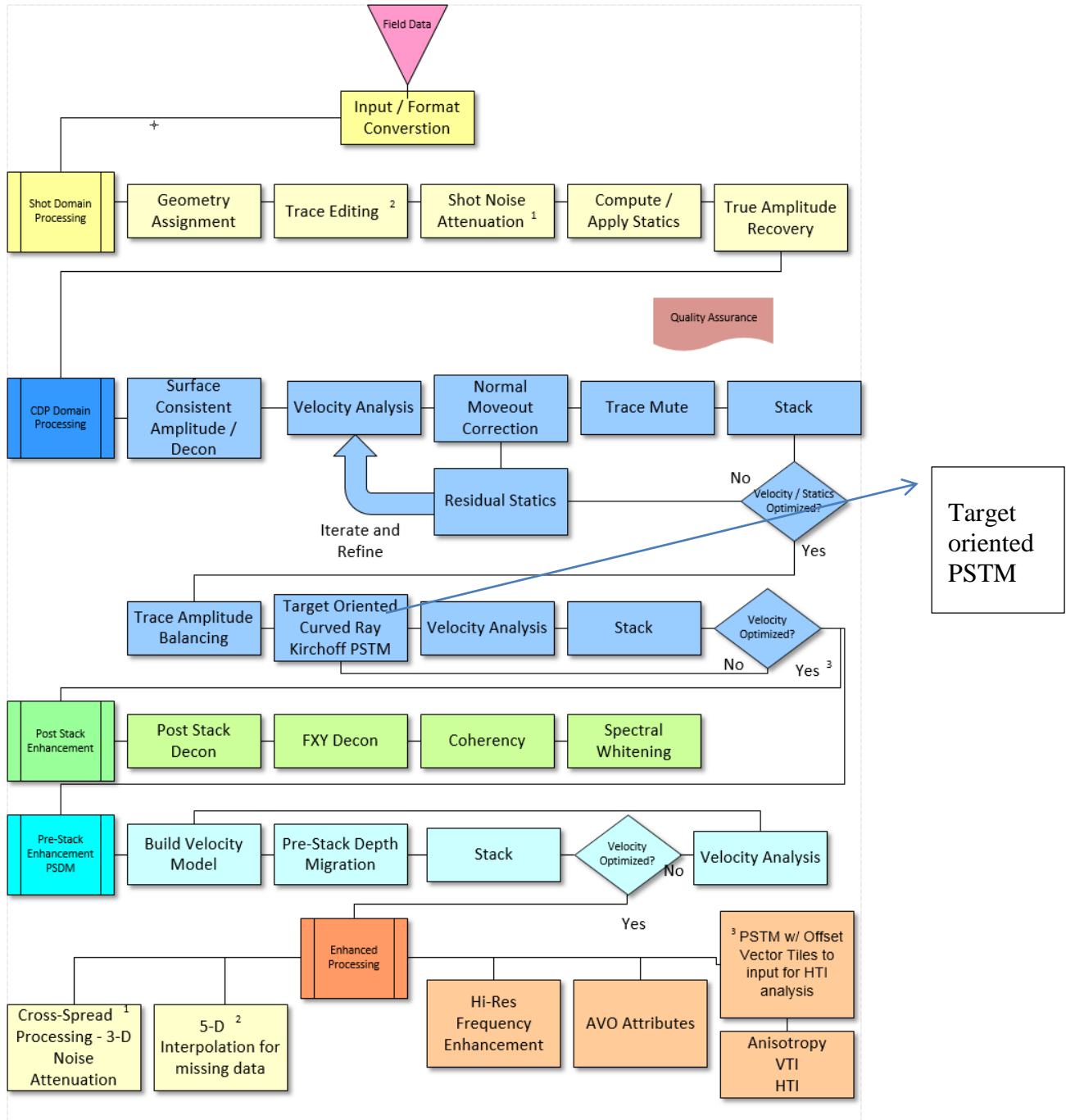
Generalised Land Seismic Processing Flow
