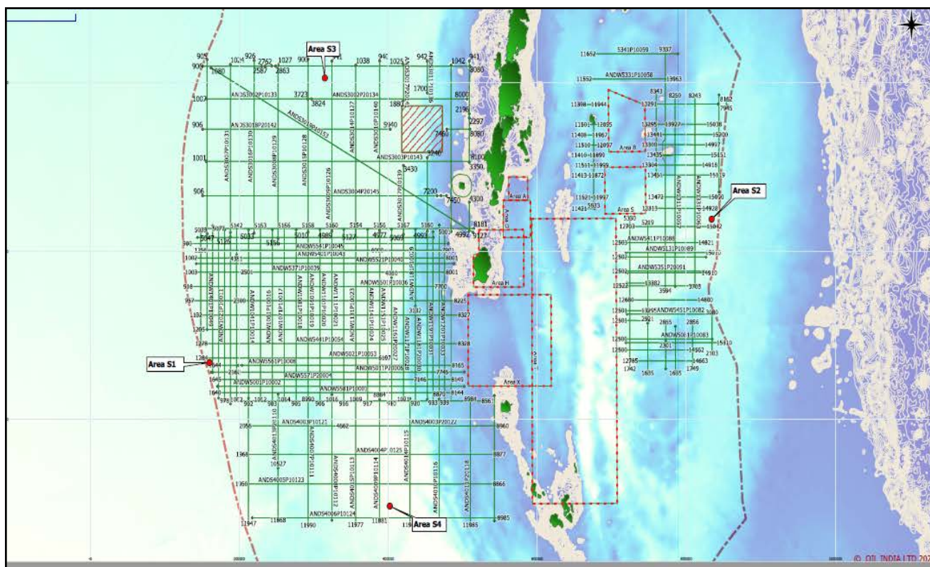
Figure 3.7: Map showing 2D seismic lines of Andaman seismic programme
